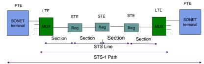
STE = Section Terminating Equipment, e.g., a repeater/regenerator
