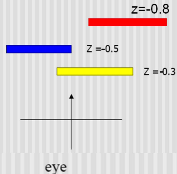
If the depth value is larger than that in the z-buffer, the pixel is coloured and value in the z-buffer is updated
