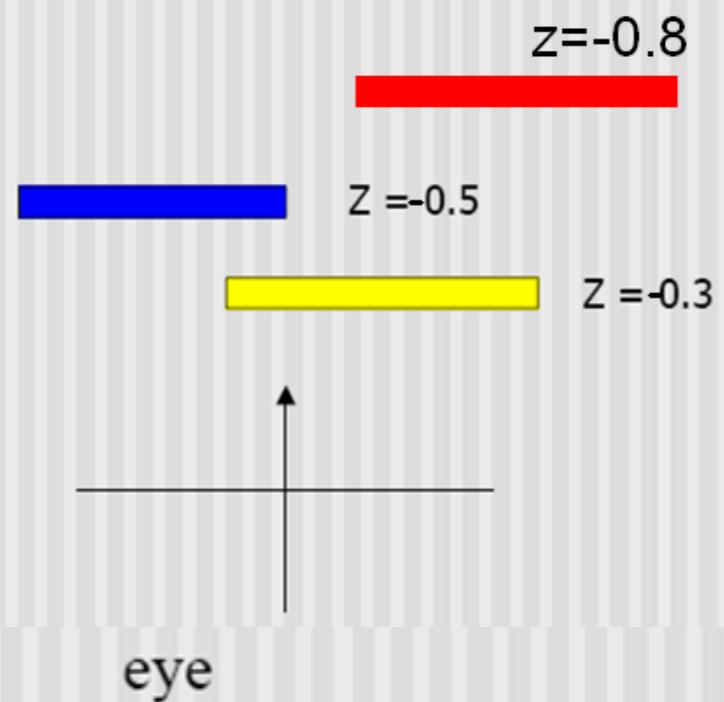
If the depth value is larger than that in the z-buffer, the pixel is coloured and value in the z-buffer is updated
