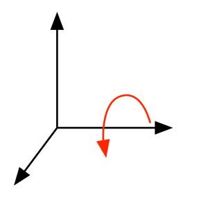
$$\begin{pmatrix} x' \\ y' \\ z' \\ 1 \end{pmatrix} = \begin{pmatrix} 1 & 0 & 0 & 0 \\ 0 & \cos \theta & -\sin \theta & 0 \\ 0 & \sin \theta & \cos \theta & 0 \\ 0 & 0 & 1 \end{pmatrix} \begin{pmatrix} x \\ y \\ z \\ 1 \end{pmatrix}$$
