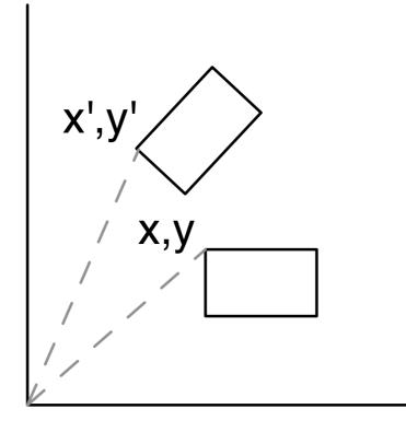
$$\begin{pmatrix} x' \\ y' \end{pmatrix} = \begin{pmatrix} \cos \theta & -\sin \theta \\ \sin \theta & \cos \theta \end{pmatrix} \begin{pmatrix} x \\ y \end{pmatrix}$$
