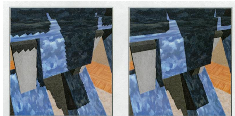
Figure 2: A conventional 2,048×2,048 pixel shadow map (left) compared to a 16 MB ASM (right). EFFECTIVE SHADOW MAP SIZE: 65,536×65,536 PIXELS.
