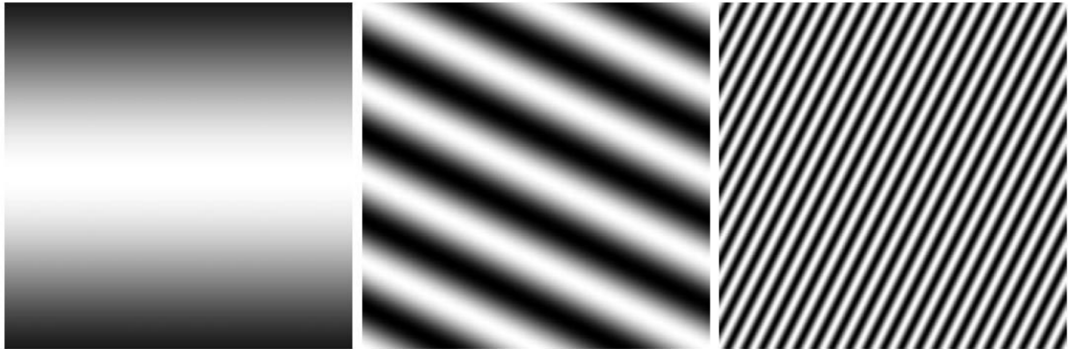
FIGURE 4.5: The real component of Fourier basis elements shown as intensity images. The brightest point has value one, and the darkest point has value zero. The domain is [-1, 1] \times [-1, 1] , with the origin at the center of the image. On the left , (u, v) = (0, 0.4) ; in the center , (u, v) = (1, 2) ; and on the right (u, v) = (10, -5) . These are sinusoids of various frequencies and orientations described in the text.
