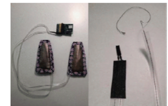
EKG sensor pads, connected to a GRASP board (A); Conductive thread insulated by scotch tape (B)
