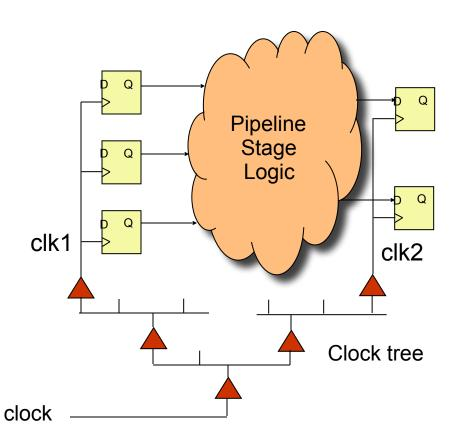
Ideally, all delays through every pipeline stage are identical
