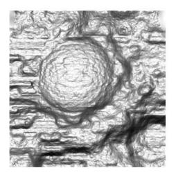
Because the wall behind the sphere is an untextured and white, the stereo system does not have much data for proper stereo matching. This explains the unusual depth data observed for the wall. On the other hand, the data from the sphere is clearly better, although still noisy.
