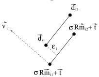
$\vec{v}_i$  is perpendicular to rotated model line i
