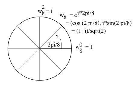
"Wheel" representation of 8th roots-of-unity (complex plane)). Same wheel structure for any n (then  $\omega_n$  found at angle  $2\pi/n$ ).
