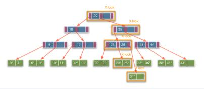
Obtain X-locks while descending; leaf-node is not safe so create a new one and lock it in X-mode; first release locks on leaves
