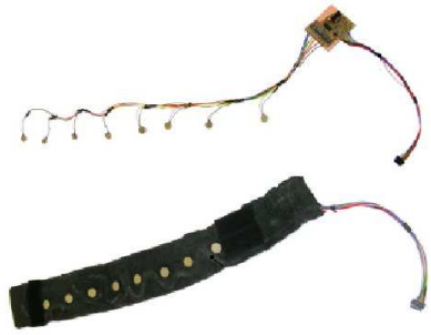
Figure 3.1: Vibrotactile array with 8 independently controlled motors, each one of which can vibrate at different frequencies (extracted from Saunders and Vijayakumar [18]).
