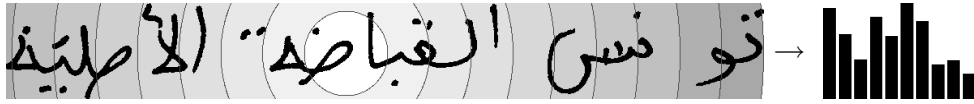
Figure 4.1: Example of the Radial Method using 10 bins. The number of pixels falling in each section form a 10-dimensional feature vector.
