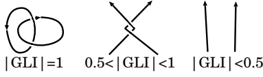
Figure 4. The GLI of directed curves when one strand is surrounding the other (left), singly tangled (middle), and untangled (right)
