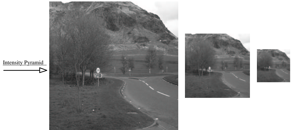
Fig. 15. The intensity pyramid built from the photograph given in Figure 13.
