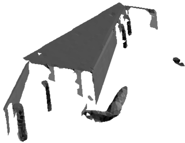
Figure 4. The constrained mesh model for the factory scene. Note how the central fold edge is straighter than in Figure 1.
