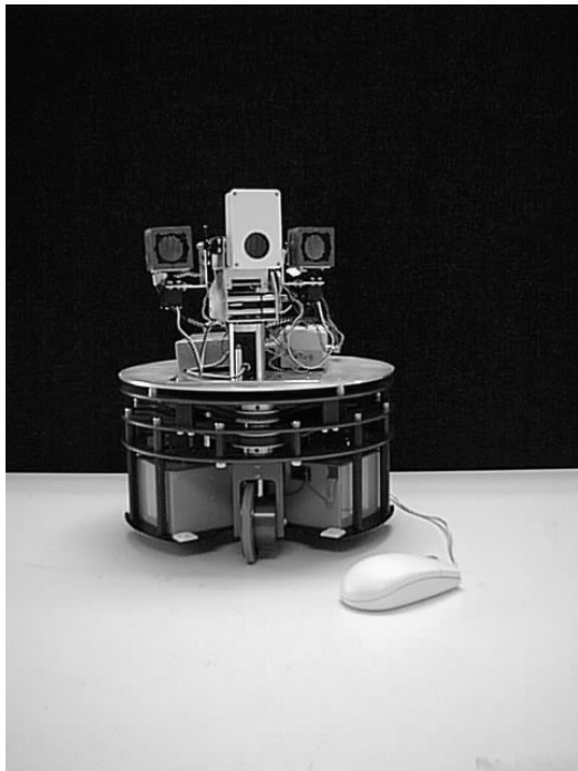
Figure 2: RoBat: a biomimetic sonarhead mounted on a mobile robot.
